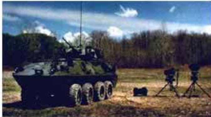
Figure 19 – Coyote LAV Reconnaissance with MSTAR Battlefield Surveillance Radar on Ground Mount (Object on Tripod to Extreme Right)
