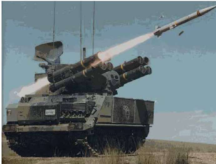
Figure 18 – CF ADATS (Its radar is used for both surveillance and tracking targets)
