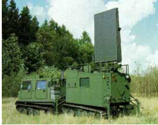
Figure 22 – Arthur Weapons Locating Radar Mounted on a Bv 206 Vehicle
