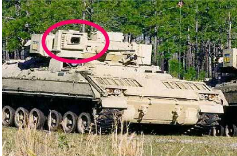
Figure 33 – Stingray Laser Dazzler Mounted on a US Army Bradley Infantry Fighting Vehicle
